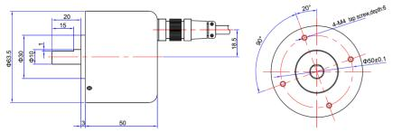
4. Connector /Dust and splash proofed with rear cable (CW type)
