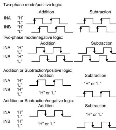
Note: The diagram above shows the assumption that the rotary encoder is rotating anti-clockwise, if the encoder is rotating clockwise, the addition diagram is adverse to the subtraction diagram.
